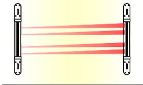
Fig. 5 – Wall mounting – Facing walls
