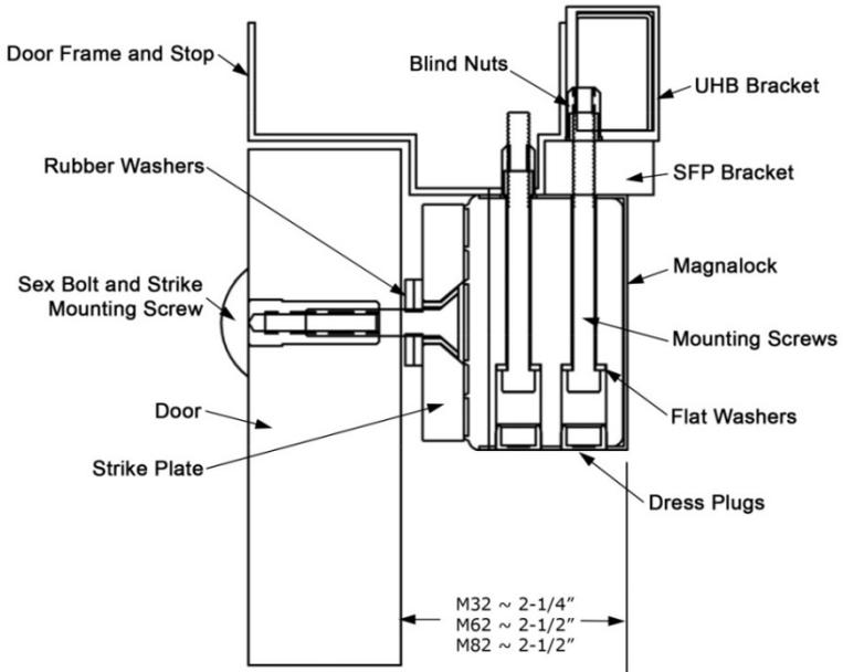
Figure 2. Magnalock Installation on an Out-Swinging Door
