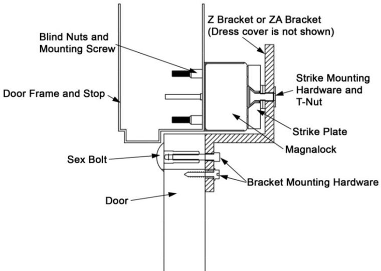
Figure 3. Magnalock Installation on an In-Swinging Door
