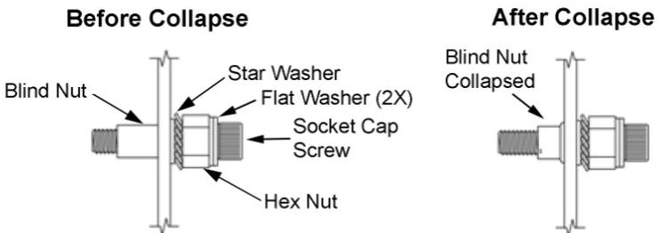
**Figure 10. Blind Nut Before and After Collapse**
