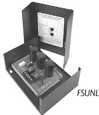
The FSUNL is used with an UNL or MUNL installation to provide selectable fail safe or fail secure behavior. Removal of power initiates a full unlatch or latch cycle depending on which mode is selected.
