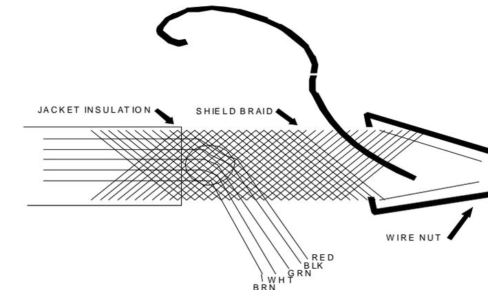
Attach an insulated #18 gauge stranded wire to the shield with a wire nut. Allow enough length for the insulated #18 wire to reach the ground lug in the back of the CAT back box.
