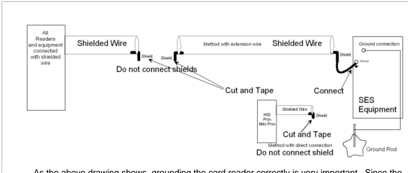
As the above drawing shows, grounding the card reader correctly is very important. Since the ground lug for the CAT is near the top of the unit, take care to avoid shorting the card reader cable shield to components on the mother board.
