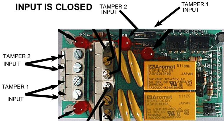
The two tamper signal inputs are "dry" contact input only. These inputs are normally open and actuate the alarm relay upon contact closure. To simplify troubleshooting in the field, an LED indicator lights whenever the input signal is closed
