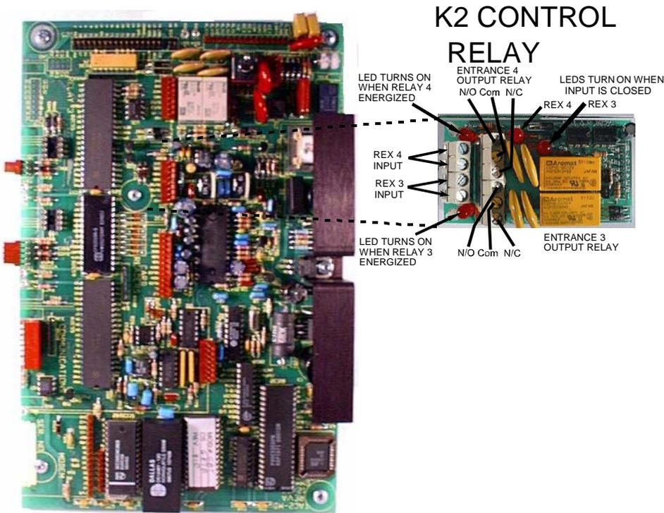
The relay capabilities are 24 volts AC or DC at 3 amps. Form "C" (N/O) AND (N/C) contacts are on the control output relay for controlling devices.
