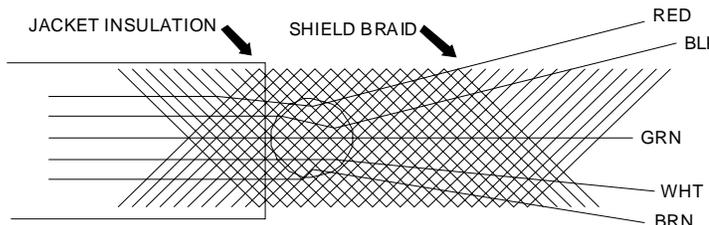
Poke a hole in the braid as shown at left. Spread the braid open, so the conductors are visible. Peel the conductors out, taking care not to damage the insulation on the conductors.
