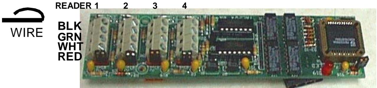
Strip 3/16" insulation from the conductors. Fold the stripped portion of the conductor over the insulated portion. Insert the wire in the clamps of the screw terminals on the card reader board and clamp down by screwing the terminal screw tightly. This ensures a good mechanical connection and an electrical connection that will keep the small wires from breaking.
