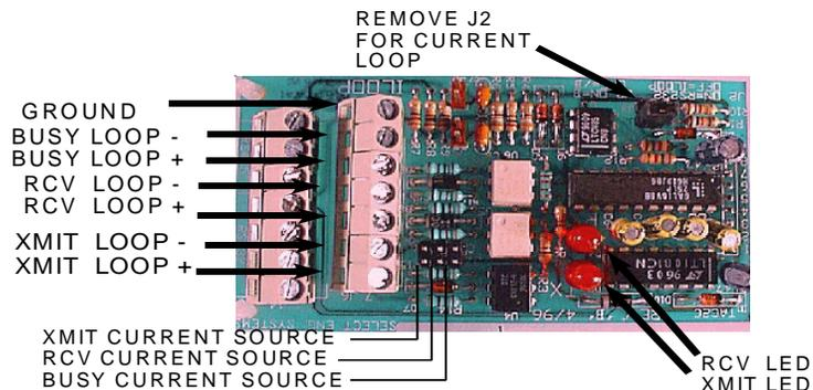
A recommended cable is Belden # 8770. The shield connects to the ground lug on the terminal barrier strip inside the CAT housing (see Pg.7).
