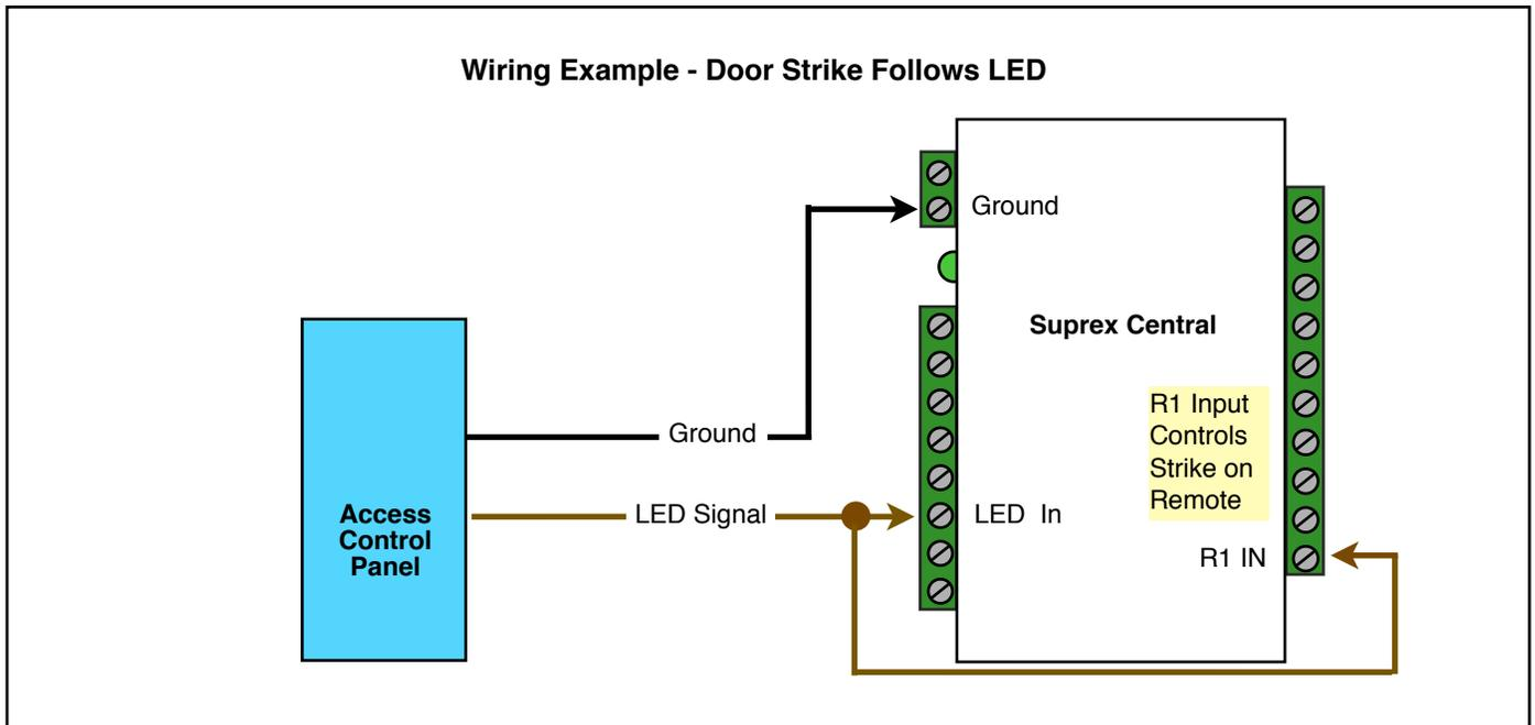
Only Relay and LED Connections are shown for clarity, refer to previous diagrams for Power and Data connections.
