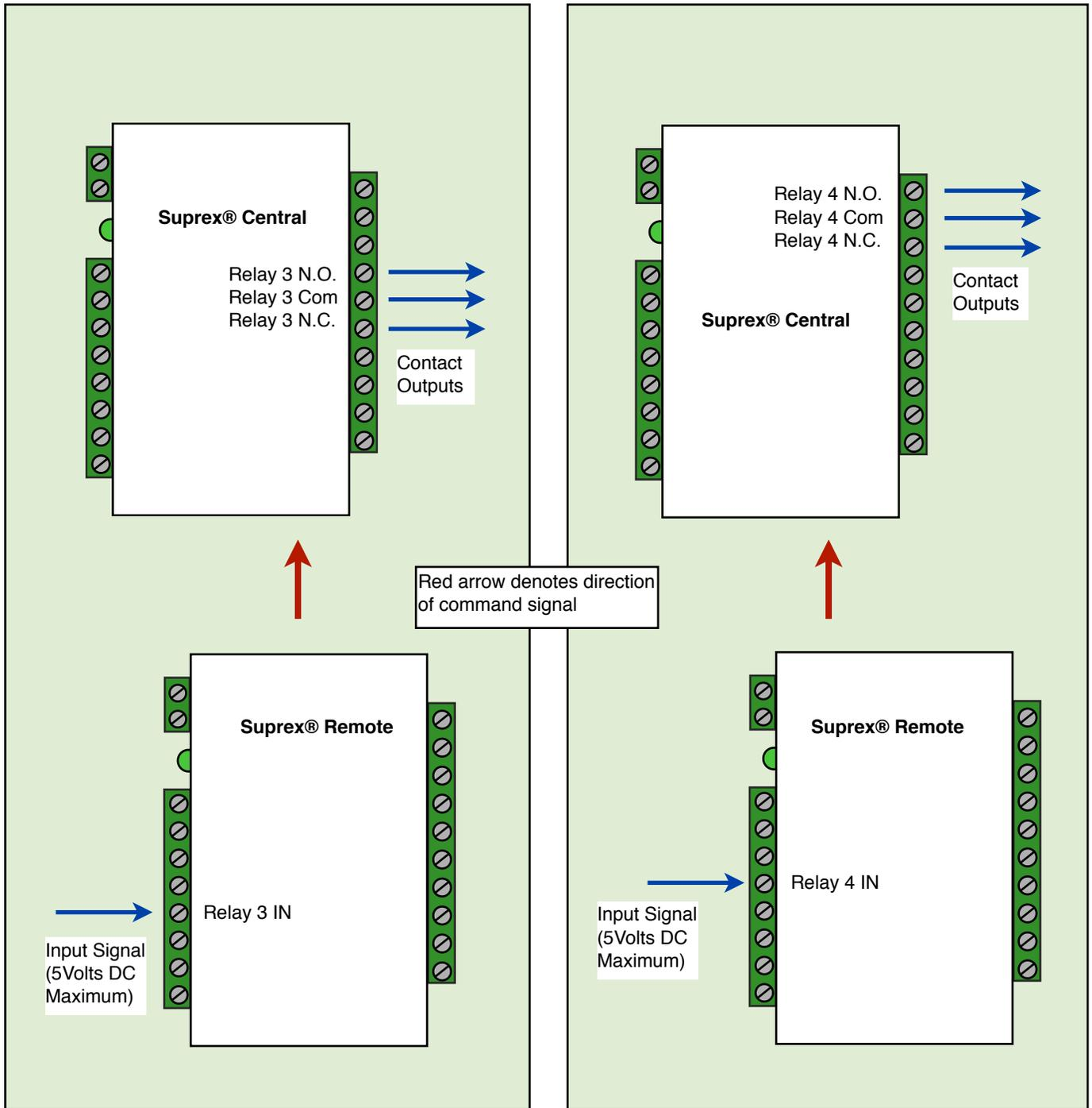
Relay 3 functions as an Alarm relay and monitors the condition of the communication link between the Central and Remote units. Relay 3 is activated when power is applied and the communication link between the Central and Remote is functioning. Relay 3 will become deactivated (Alarm condition) when either the Relay 3 input on the remote is active OR the Remote unit is unable to communicate with the Central unit. See APP NOTE FOR DETAILS
