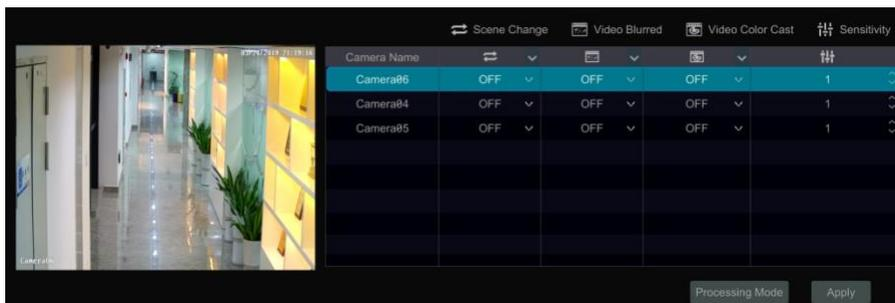
② Select the camera and enable the relevant detection as needed.
