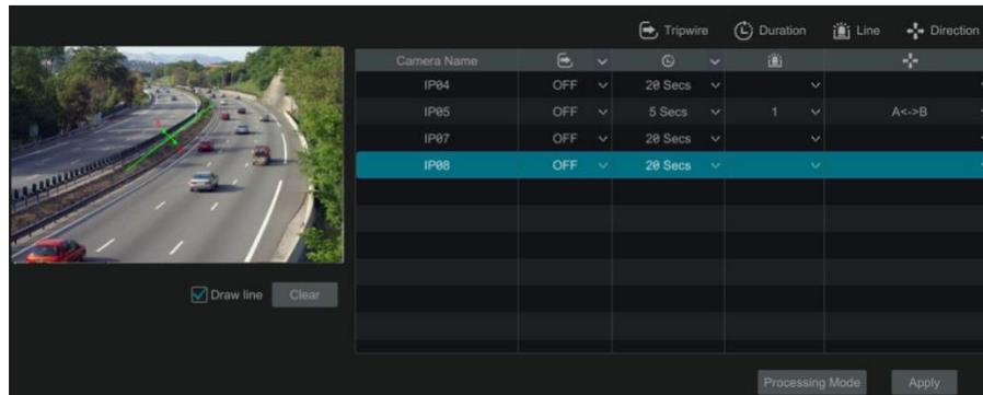
② Select the camera, enable the line crossing detection.
