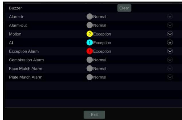
Click “Clear” to stop the buzzer when the buzzer alarm happens. Click
