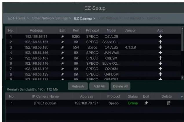
Click to edit the searched IP camera as shown on the below left. Enter the new IP address, subnet mask, gateway, username and the password of the camera. You can check “Sync to IPC” to modify the IP address of the IPC via different network segments for being in the same network segment with the NVR. Click “OK” to save the settings.
