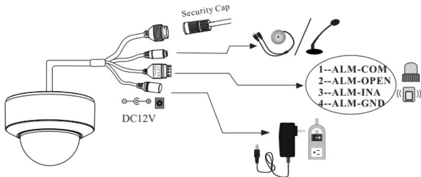
**\* 1 It is recommended to install the security cap for outdoor installations.**
