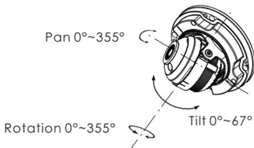
⑥ Install the lower dome back to the camera and fasten it with the screws. Then put the trim ring onto the lower dome and then rotate it clockwise until it is locked.
