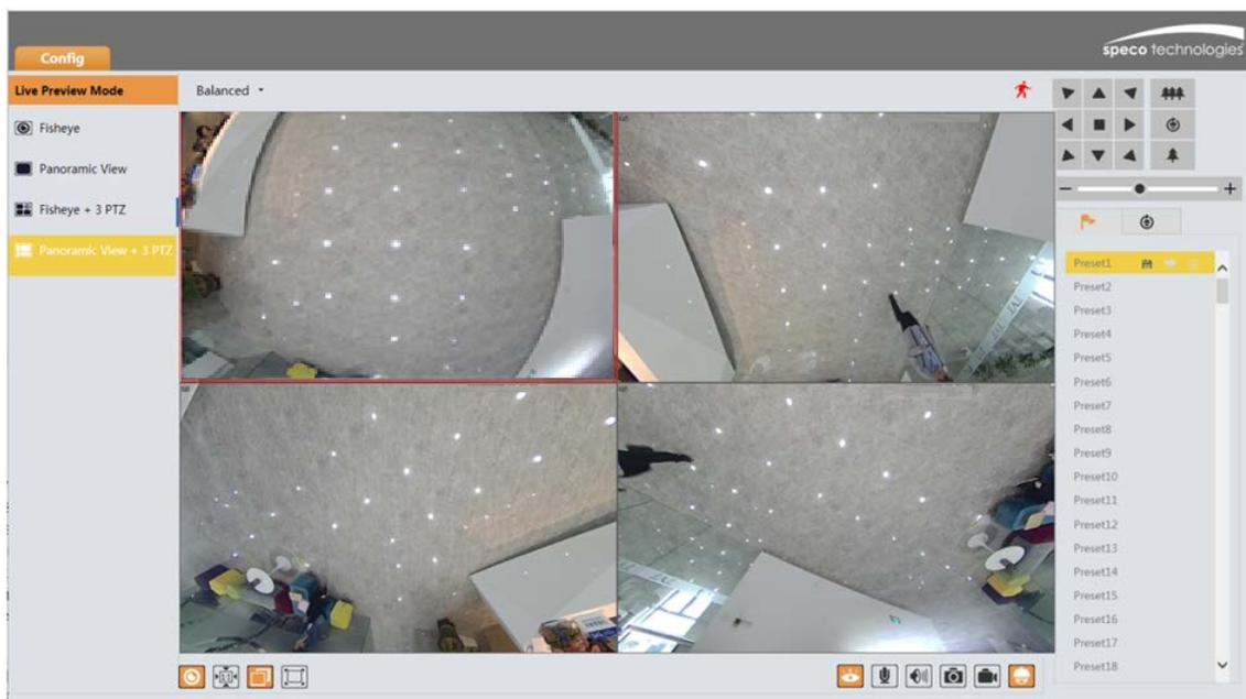
**4PTZ view mode** (you need to switch the stream mode in the fisheye parameter interface)
