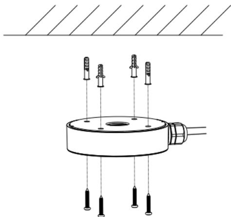
③ Route the cables through the cable hole (take side conduit cabling for example) and connect the cables. Then fix the camera onto the junction box with screws.
