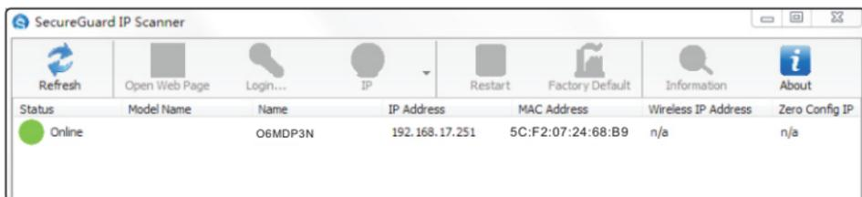
③ In the device list, you can view the IP address, model number, and MAC address of each device. Select the applicable device and double click to open the web viewer. You can also manually enter the IP address in the address bar of the web browser.
