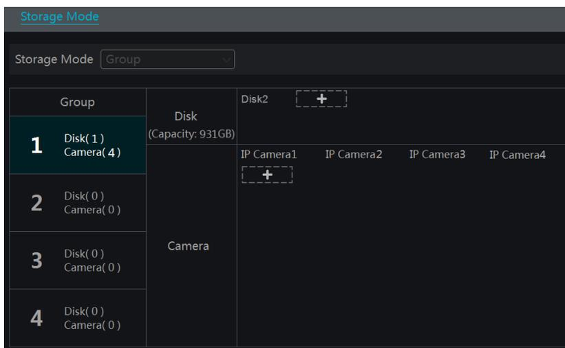
There are all four disk groups. By using disk group, you can correspond the camera to disk (the record data of the camera in the group will be stored into the disks in the same group). The NVR with e-SATA interface supports e-SATA recording.
