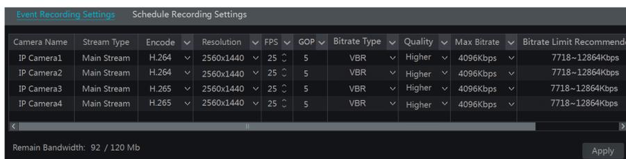
Click Start→Settings→Record→Stream Settings to go to “Sub-stream” interface. Set the encode, resolution, FPS, GOP, bitrate type, quality and max bitrate of sub-stream for each camera in the interface and then click “Apply” to save the settings.
