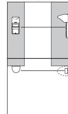
\* The sensor and reflector units should be installed uprightly and vertically. Make sure that the reflector's front side faces the sensor as illustrated.
