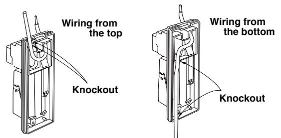
⑤ After wiring is completed, adjust alignment, attach cover and check operation. (Note : Sealing is not required around the unit due to rain-proof construction.)
