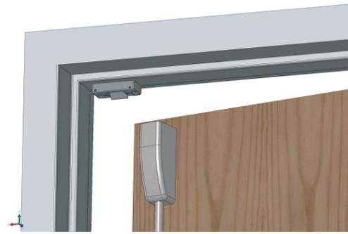
Twist off the center tab of the mounting tab, pass the plate through the mechanism hole, secure the plate using the #6-32 screws (included).
