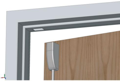
Cut the door frame header for the electric strike mechanism and drill the frame for the mounting screws
