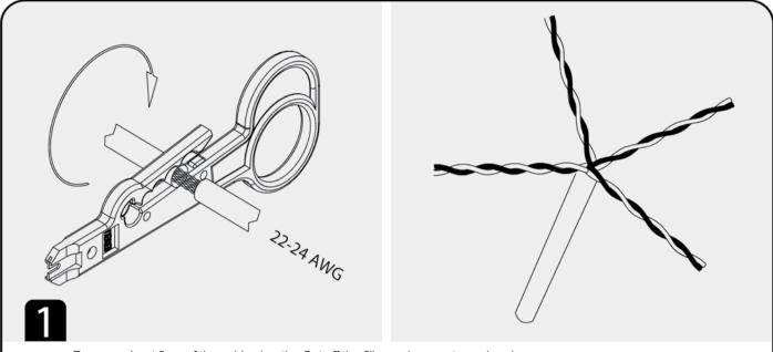
Remove about 3cm of the cable sheath. Cut off the filler and separate each pair.
