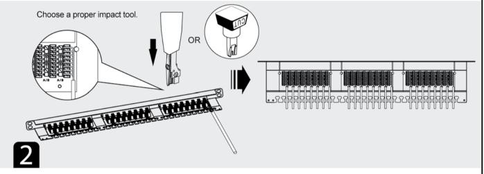
Seat each wire into the the IDC slots according to the color scheme. Punch down each wire with a proper impact tool .
