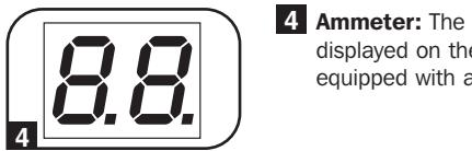
**4 Ammeter:** The total electrical current used by the PDU will be displayed on the digital meter in amperes (applies only to models equipped with an ammeter).
