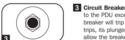
**3 Circuit Breaker:** If the current drawn by the equipment connected to the PDU exceeds the Maximum Current Rating, the circuit breaker will trip to prevent possible damage. When a circuit breaker trips, its plunger will pop up. Disconnect excess equipment and allow the breaker to cool at least one minute before depressing the plunger to reset the breaker.
