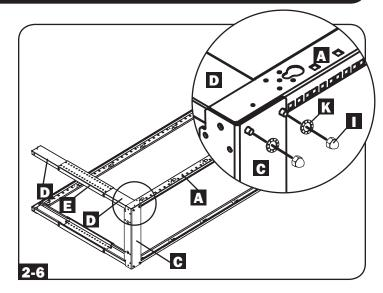
Fasten an assembled top section F/G/F to the top bracket and left vertical rail with an M8 acorn/cap nut and M8 washer .
