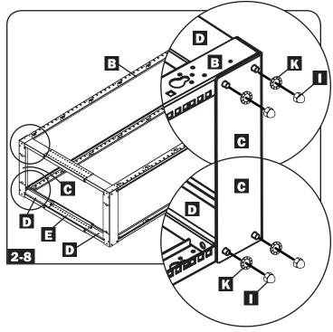
Fasten a top bracket to the threaded M8 stud at the end of the assembled top section f/G/F with an M8 acorn/cap nut and M8 washer . Also fasten the base bracket to the threaded M8 stud at the end of the other assembled bottom section with an M8 acorn/cap nut and M8 washer . Tighten 90%. (The threaded M8 studs should pass through the vertical rails first, then the top bracket.)
