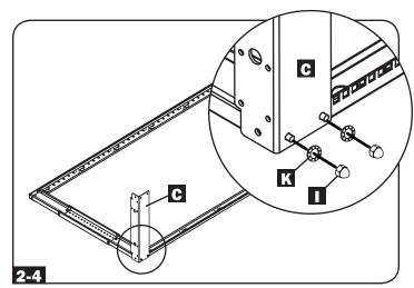
at the end of the assembled top section with an M8 acorn/cap nut ■ and M8 washer ₭. Tighten 90%. (The threaded M8 stud should pass through the vertical rail first, then the top bracket.)
