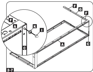
Fasten a base bracket G and right vertical rail
