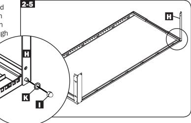
Pasten a left vertical rail A and assembled bottom section D/E/D to the base bracket with two M8 acorn/cap nuts ■ and M8 washers II. Tighten 90%. (The threaded M8 studs at the end of the assembled bottom section should pass through the vertical rail first, then the base bracket.)
