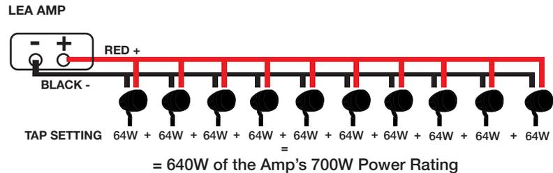
**NOTE:** If using 70V, the Acoustiscape speakers MUST be set to the proper TAP setting prior to connecting it to the amplifier. The speaker will blow if set to 8Ω and will not be covered by warranty. The higher the TAP setting the more power it will receive from the amplifier and the louder the speaker will go. The TAP settings gives the listener greater flexibility for layout design. It also allows each speaker to be tapped at different levels creating an even sound stage.
