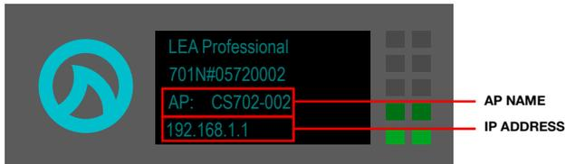
4. On a WiFi enabled device, search the available WiFi connections for the "AP Name." Select the WiFi address and connect to it on your device.
