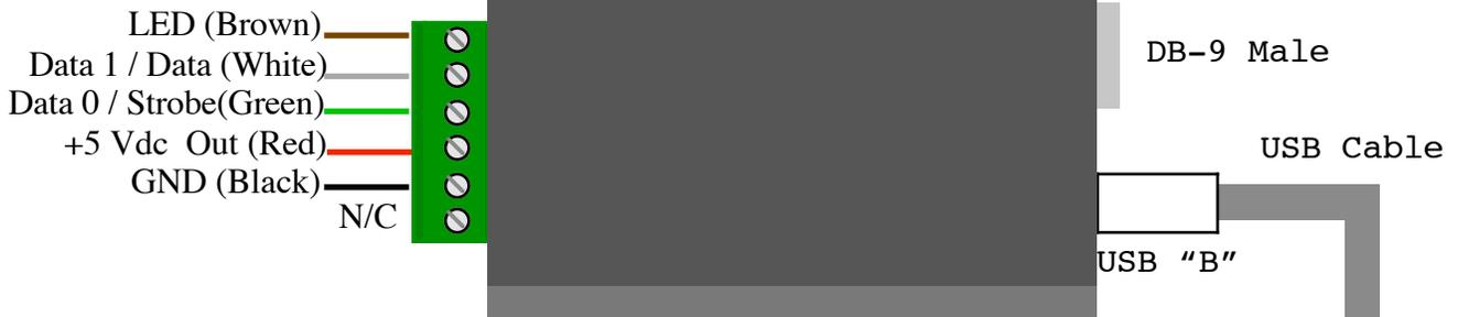
Supply Voltage: 5 Vdc from USB Interface
