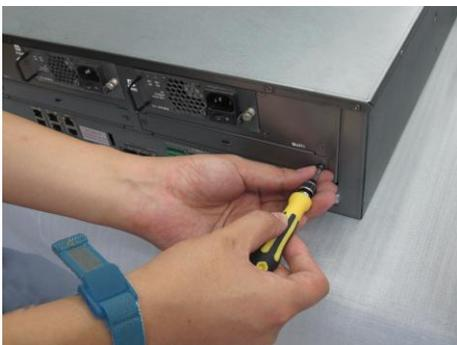
2. Insert the decoding card in place.
