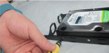
2. Unscrew the front panel with a Phillips screwdriver.
