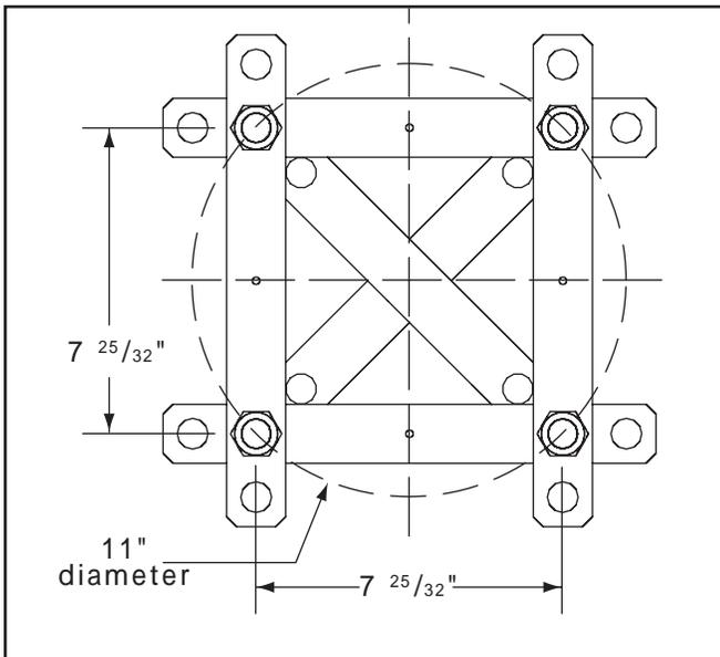
4. Before using the Anchor Jig verify that the center to center dimensions between the bolts are even (Figure 4). If not, adjust accordingly. Firmly tighten all Hex Nuts.
