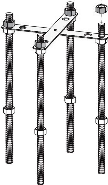
2. Place the short end of each Bolt into the outside holes of the Cross Strap. Place Hex Nuts onto each Bolt and finger tighten (Figure 2).
