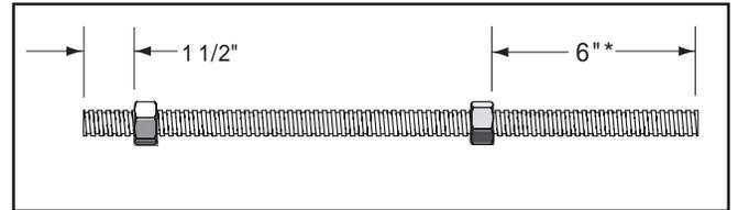
1. Thread two (2) nuts onto each of the (4) bolts (Figure 1). The end with 6" of clearance will be the top of the Anchor Jig, the end with 1 1/2" clearance will be the bottom.
