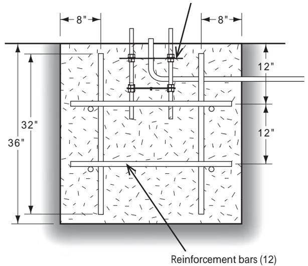
To help reinforce the concrete foundation, place (12) 1/2" diameter x 32" long Reinforcement Bars ("rebar") as shown in figure 2. Use suitable preparation methods to place the rebar.
