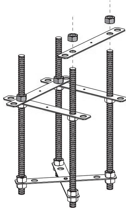
3. Turn the Anchor Jig over and place Single Straps over the Bolts (Figure 3). Use the inside hole of each strap. Place Hex Nuts onto each Bolt and finger tighten.
