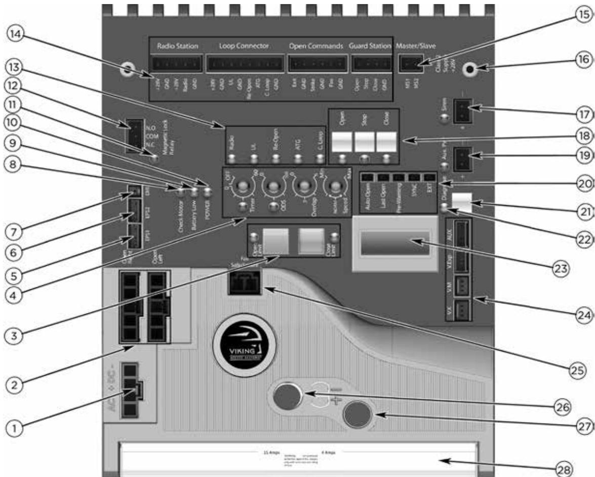
1. POWER HARNESS CONNECTOR provides power to the control board. pg 20
