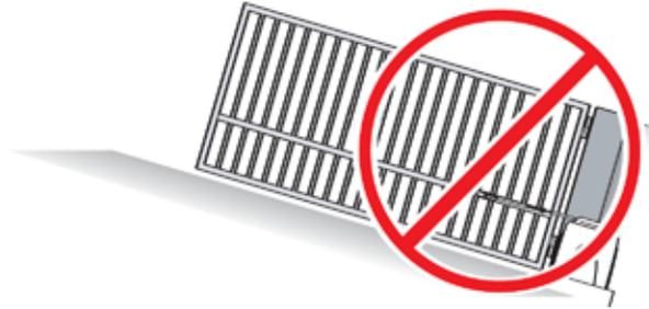
**DO NOT** install the gate operator to lift gates
