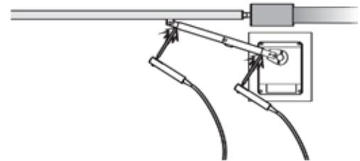
**⚠ TIP:** Use C-clamps or tack-weld the Arm assembly in place until Step 3 has been completed.
