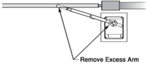
**⚠ TIP:** Leave some additional material when cutting the Arm Assembly to allow for adjustment.
