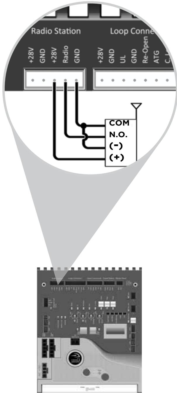
The control board provides two modes of operation that a radio receiver can control the gate:
