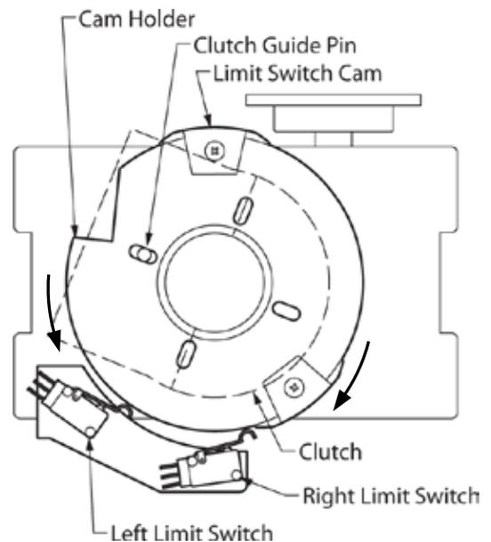
**Tip:** Referring to Step 2b. The “Cam Holder” contains four (4) Guide Pin holes to allow for proper positioning, if required, due to an alternative operator orientation.
