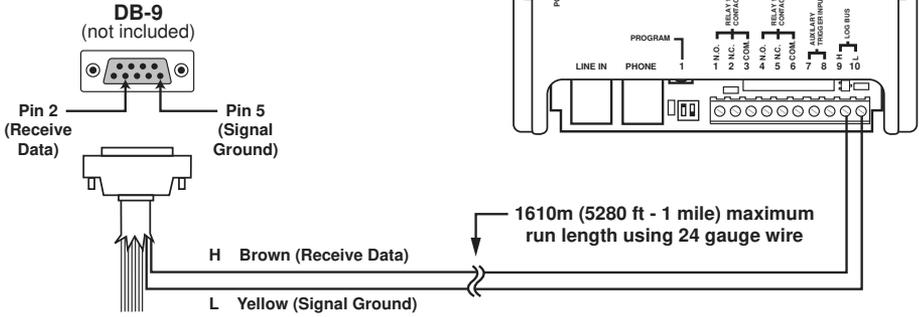
If the RS-232 input of a PC, printer, etc. is capable of receiving TTL level RS-232 signals, then the **LOG BUS** can be wired directly into the RS-232 "Receive Data" and "Signal Ground" pins to receive ASCII data. Windows "Hyper-Terminal" can be used to receive the data on a PC (use the settings in the chart) or visit [www.vikingelectronics.com](http://www.vikingelectronics.com) to download free ENTRY LOGGER software (see **Operation** section E, "Entry Logger Software").
