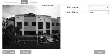
Set the alarm area number and then input the alarm area name on the right side. You can add 4 alarm areas at most.
