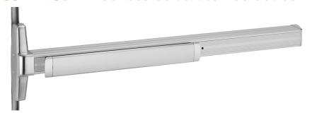
**3347A** and **3547A** for all types of single and double doors, UL listed for panic exit hardware. Devices are ANSI A156.3 – 2008 Grade 1. The 3547A has a smooth mechanism case and the 3347A has grooved case. The concealed vertical rod device is non-handed except when the SS (signal switch) option is used. See opposite page for available outside trim and device functions.
