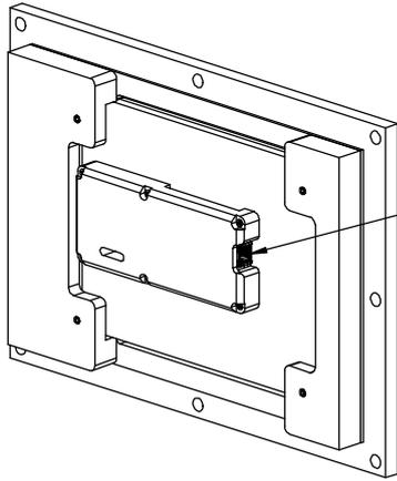
Before installation of the wall mount, connect a 48V IEEE 802.3at POE+ power source via a CAT5/6 cable and RJ45 connector to the POE to USB converter.
