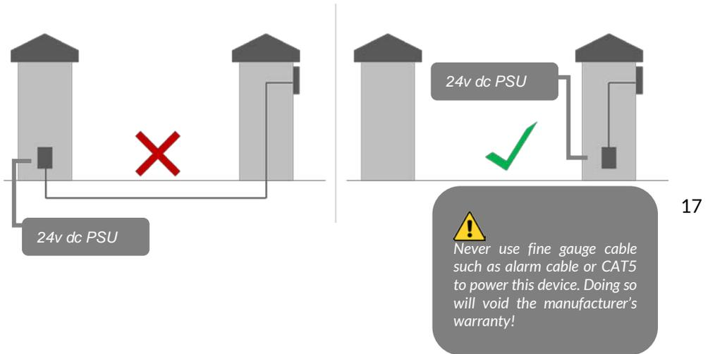
Up to 2 meters (6 feet) use minimum 0.5mm / 18 gauge cable.
