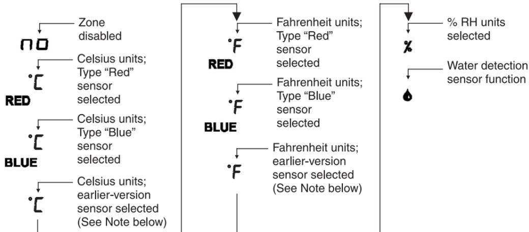
**Note:** Sensor types ("Red", "Blue" or plain °F or °C) refer to the Zone programming required for the type of sensor used:
